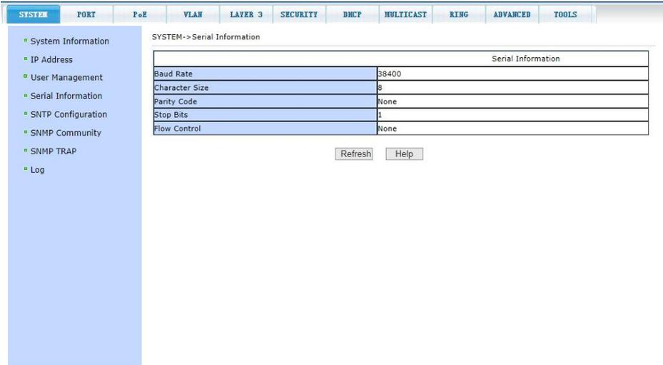
The screenshot shows a web interface with a navigation menu on the left and a main content area. The navigation menu includes: System Information, IP Address, User Management, Serial Information, SNMP Configuration, SNMP Community, SNMP TRAP, and Log. The main content area is titled 'SYSTEM-> Serial Information' and contains a table with the following data:
