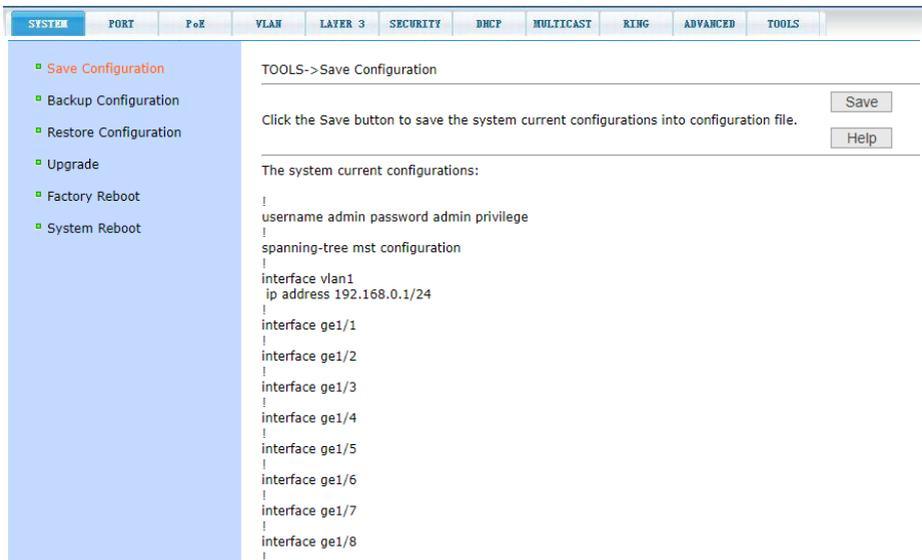
The screenshot shows a web interface with a top navigation bar containing tabs: SYSTEM, PORT, PoE, VLAN, LAYER 3, SECURITY, DHCP, MULTICAST, RING, ADVANCED, and TOOLS. The 'TOOLS' tab is active. On the left, a sidebar menu lists: Save Configuration (highlighted), Backup Configuration, Restore Configuration, Upgrade, Factory Reboot, and System Reboot. The main content area is titled 'TOOLS -> Save Configuration' and contains the following text and elements:
