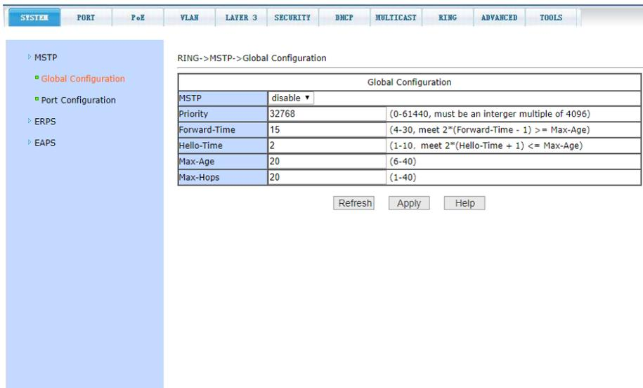
The screenshot displays the configuration page for MSTP in the RING environment. The navigation menu on the left includes SYSTEM, PORT, PoE, VLAN, LAYER 3, SECURITY, DHCP, MULTICAST, RING, ADVANCED, and TOOLS. The main content area is titled 'RING->MSTP->Global Configuration' and contains a table of settings for 'Global Configuration'.
