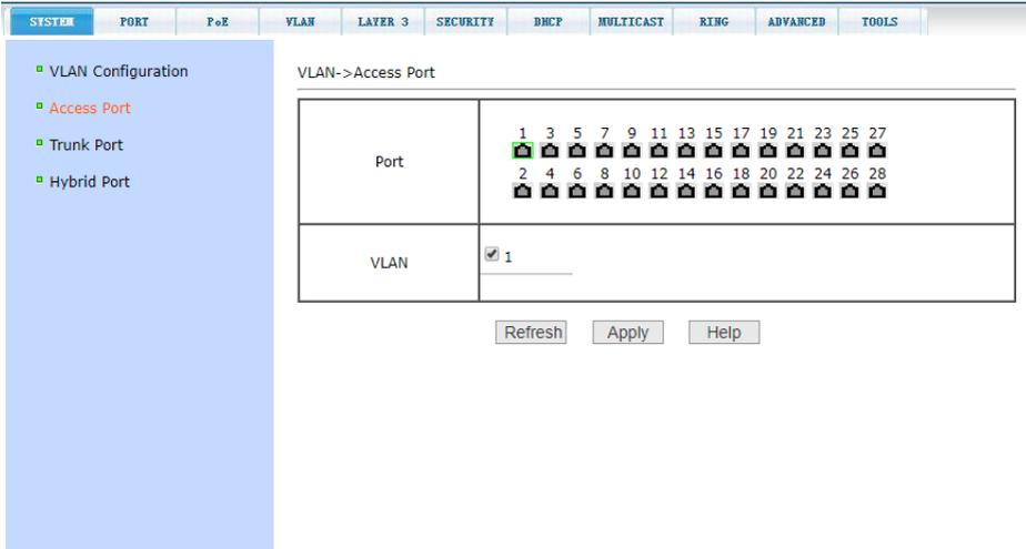
The screenshot displays the 'VLAN->Access Port' configuration page. On the left, a navigation menu lists 'VLAN Configuration', 'Access Port', 'Trunk Port', and 'Hybrid Port'. The main content area features a grid of 28 ports, arranged in two rows of 14. Each port has a checkbox and a small icon. The first port in the first row is selected. Below the grid, a 'VLAN' field contains a dropdown menu with '1' selected. At the bottom, there are three buttons: 'Refresh', 'Apply', and 'Help'.
