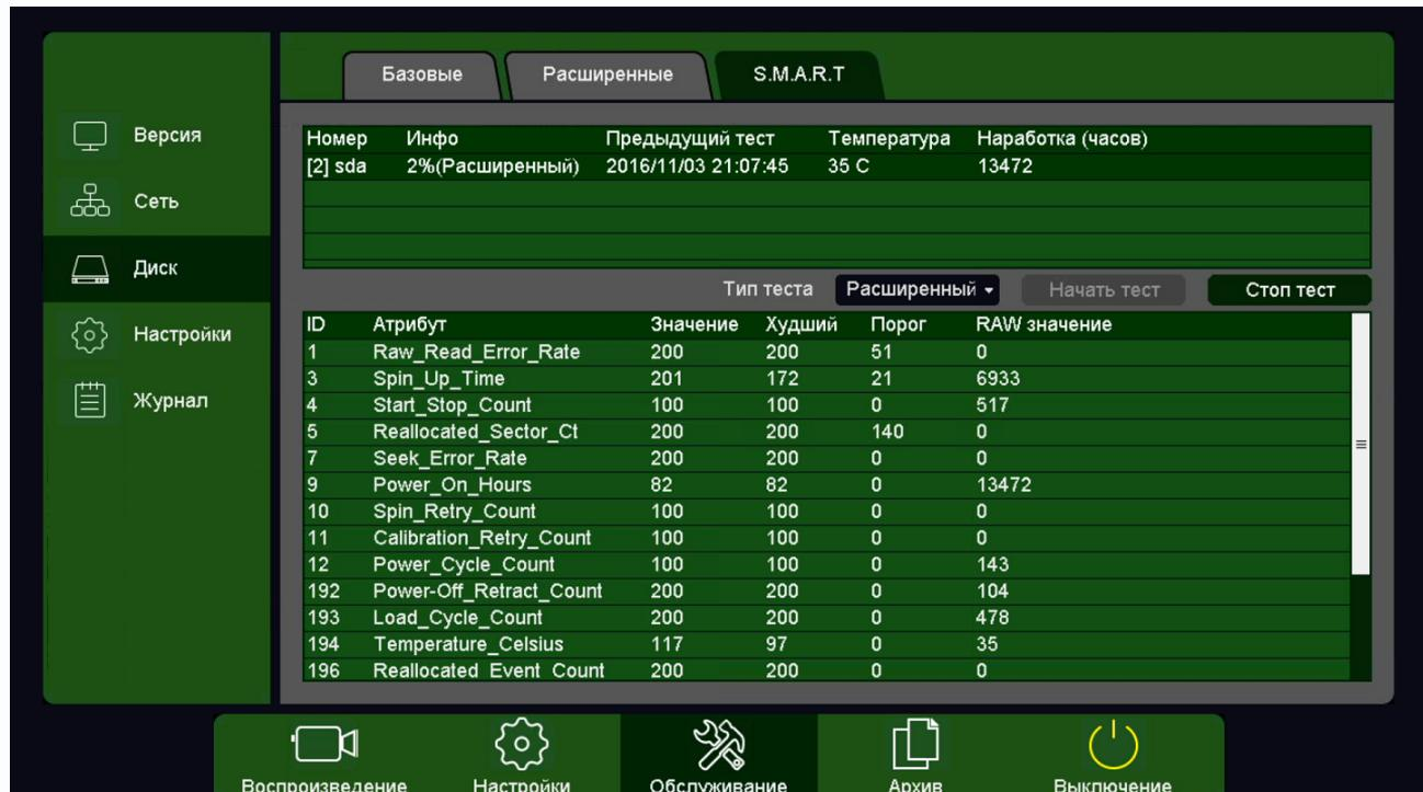
The screenshot shows the software interface for managing disk tests. On the left is a vertical menu bar with icons for Version, Network, Disk, Settings, and Log. The main window has three tabs at the top: Базовые (Basic), Расширенные (Advanced), and S.M.A.R.T. The Advanced tab is selected. Below it is a table with disk information:
